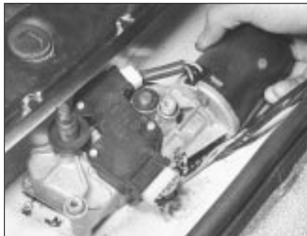
25.5B Removing windscreen wiper motor
