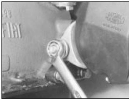
4.2A Alternator mounting
