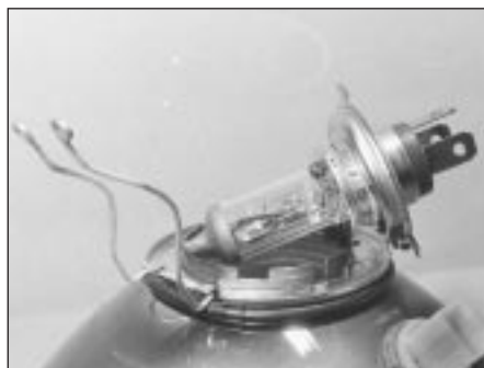
16.2B Headlamp halogen type bulb
