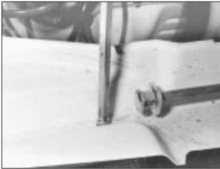
18.1 Headlamp upper fixing screw
